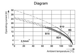
The illustration shows the derating diagram of various series B contact inserts (B6 to B24), conductor cross section 2.5 mm²
