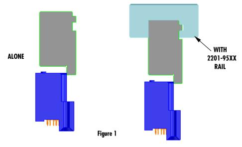
The 62201-95XX rail is available in a variety of lengths to accommodate multiple press-in tools:
