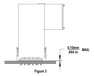
There should be no broken stand-offs along the perimeter of the part (an indication of over-pressing).
