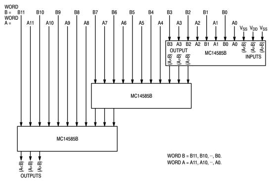
Figure 3. Cascading Comparators
