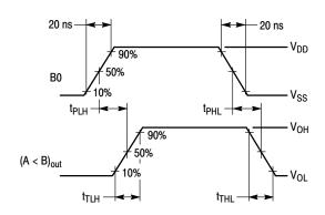
Inputs (A>B) and (A=B) high, and inputs B3, A3, B2, A2, B1, A1, A0, and (A<B) low.
