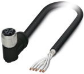
Sensor/Actuator cable, 5-position, PE-X halogen-free, black, shielded, free cable end, on Socket angled M12 SPEEDCON, A-coded, Cable length: 2 m, For railway applications
