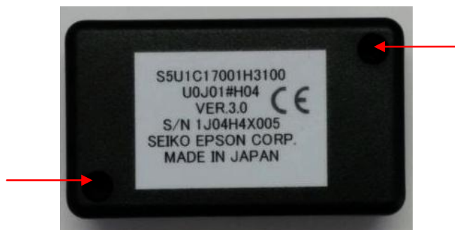
Figure 5.1 Screw Positions on the Bottom Cover
