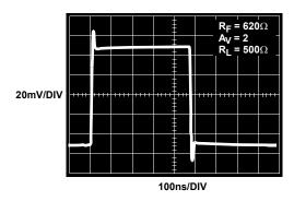
FIGURE 18. SMALL SIGNAL STEP RESPONSE (V<sub>S</sub> = ±2.5V)
