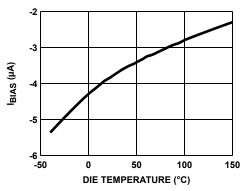
FIGURE 34. INPUT BIAS CURRENT vs TEMPERATURE
