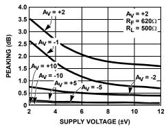
FIGURE 14. PEAKING vs SUPPLY VOLTAGE
