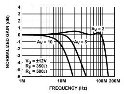
FIGURE 3. NON-INVERTING FREQUENCY RESPONSE (GAIN)
