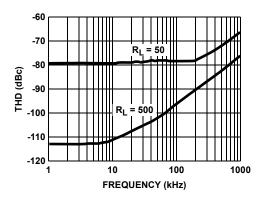
FIGURE 28. TOTAL HARMONIC DISTORTION vs FREQUENCY @  $2V_{P-P}$   $V_S = \pm 2.5V$
