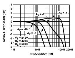
FIGURE 4. INVERTING FREQUENCY RESPONSE (GAIN)
