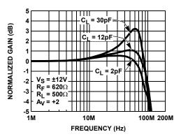
FIGURE 9. NON-INVERTING FREQUENCY RESPONSE FOR VARIOUS  $C_{L}$
