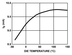
FIGURE 32. SUPPLY CURRENT vs TEMPERATURE
