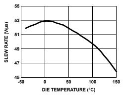
FIGURE 35. SLEW RATE vs TEMPERATURE
