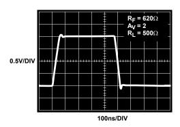
FIGURE 16. LARGE SIGNAL STEP RESPONSE ( $V_S = \pm 2.5V$ )
