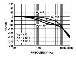
FIGURE 5. NON-INVERTING FREQUENCY RESPONSE (PHASE)
