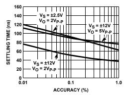
FIGURE 36. SETTLING TIME vs ACCURACY
