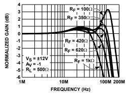
FIGURE 2. INVERTING FREQUENCY RESPONSE FOR VARIOUS  $R_{\rm F}$
