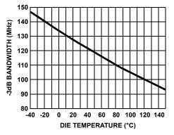
FIGURE 31. -3dB BANDWIDTH vs TEMPERATURE
