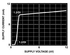
FIGURE 21. SUPPLY CURRENT vs SUPPLY VOLTAGE
