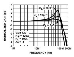
FIGURE 10. INVERTING FREQUENCY RESPONSE FOR VARIOUS  $\mathbf{C}_{L}$
