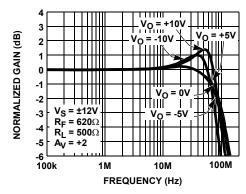
FIGURE 12. FREQUENCY RESPONSE FOR VARIOUS OUTPUT DC LEVELS
