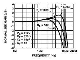
FIGURE 11. NON-INVERTING FREQUENCY RESPONSE FOR VARIOUS  $\mathbf{R}_{L}$
