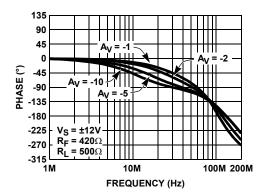
FIGURE 6. INVERTING FREQUENCY RESPONSE (PHASE)
