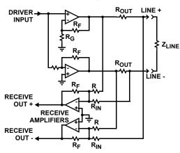
FIGURE 38. TYPICAL LINE INTERFACE CONNECTION
