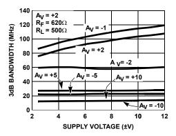
FIGURE 13. 3dB BANDWIDTH vs SUPPLY VOLTAGE
