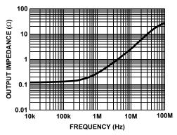
FIGURE 22. CLOSED LOOP OUTPUT IMPEDANCE vs FREQUENCY
