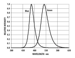
Figure 5. Relative Intensity vs Wavelength
