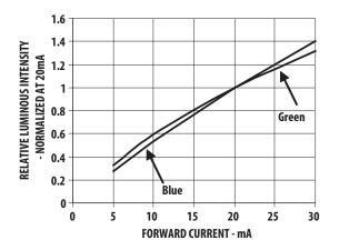
Figure 7. Relative Intensity vs Forward Current
