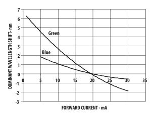
Figure 9. Relative dominant wavelength vs Forward Current
