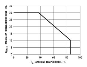
Figure 8. Maximum Forward Current vs Ambient Temperature
