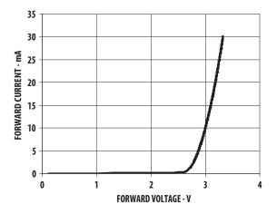
Figure 6. Forward Current vs Forward Voltage
