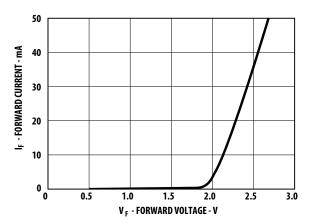
Figure 3. Forward Current vs Forward Voltage
