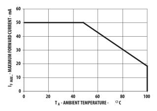
Figure 2. Maximum Forward Current vs Ambient Temperature
