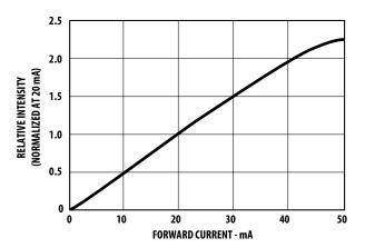
Figure 4. Relative Intensity vs Forward Current
