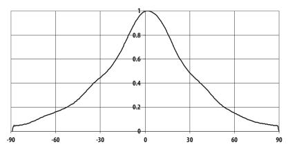
Figure 11. Radiation pattern-Minor Axis
