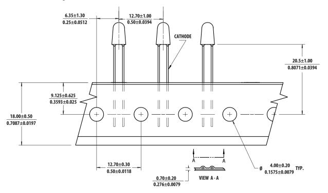
$Note: The\ ammo-packs\ drawing\ is\ applicable\ for\ packaging\ option\ -DD\ \&\ -ZZ\ and\ regardless\ standoff\ or\ non-standoff\ or\ no$
